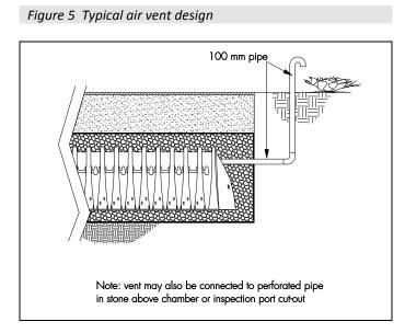
8.2 As a minimum, one 110 mm diameter air vent per 7500 m<sup>2</sup> of impermeable catchment area to be drained is generally sufficient. Venting should be positioned in a non-trafficked area, where possible.
