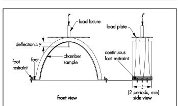
Figure 4 Arch stiffness constant test apparatus
