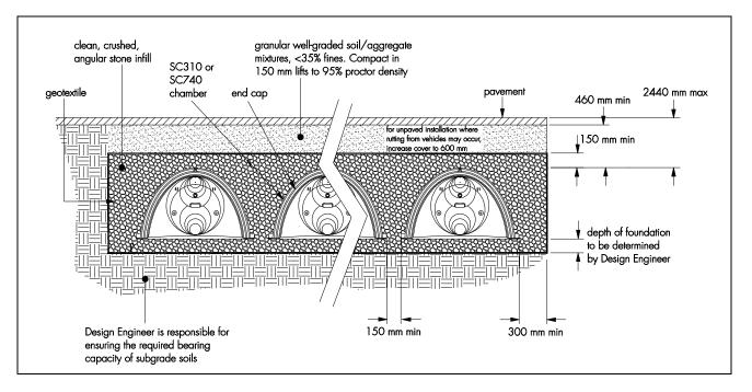
6.5 All foundation and infill stone to 150 mm above the crown of the chambers must be nominal 200 to 400 mm, clean, crushed stone in accordance with BS EN 13242 : 2013, sizes 20/40 or 20/32. Recycled crushed concrete may be an acceptable fill material but its use is outside the scope of this Certificate. Further details may be obtained from the Certificate holder.
